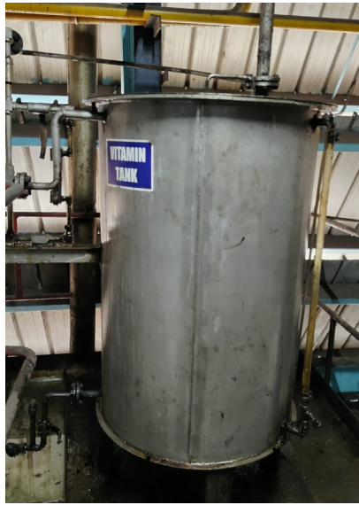
Picture: Dosing equipment for vitamin A and D in one of Kaleesuwari's oil processing plants
